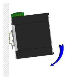
To install the unit to 35mm industrial DIN rail, place the top edge of the included mounting bracket on the back of the unit against the DIN rail at a  $15^{\circ}$  angle as shown. Rotate the bottom of the unit to the back (away from you) until it snaps into place.
